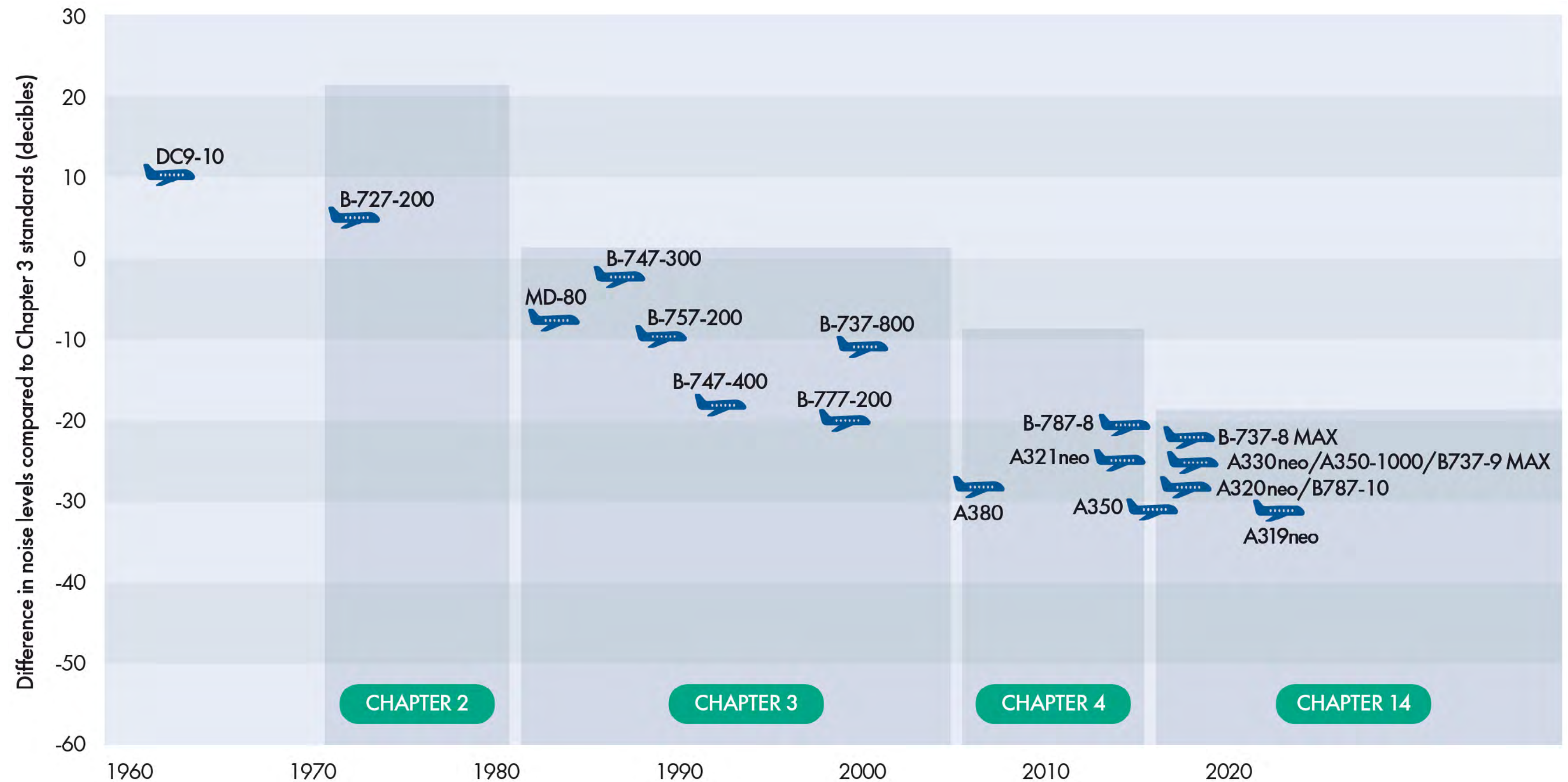
Figure 10. Downward trend in the noise certification of aircraft (Source: ICAO noise database 3 )
